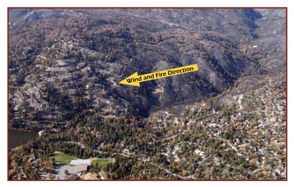
Figure 12. Consecutive burned homes where streets were aligned with the wind are indicated by the arrow. Figure 13. Typical fuels below homes on Trinity Drive and Merced Lane.
