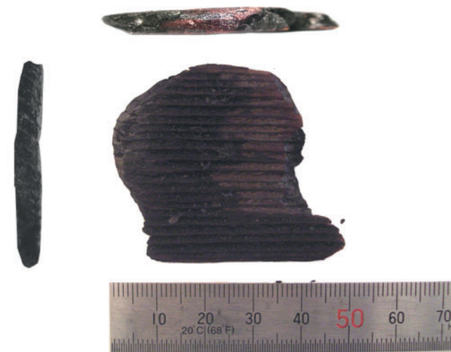
Fig. 1. A firebrand from the Oakland Hills Conflagration: ~50-mm diameter, ~5-mm thickness and 2.3 g (density of \sim 250 \text{ kg m}^{-3} ). The firebrand is presumed to have been produced from a cedar shingle (Koo et al. 2010).
